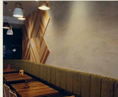
Natural renders are often thought of as a traditional building material, but Rockcote, a New Zealand-owned company that manufactures earthen renders from clay and lime, has rethought the application for contemporary use.
